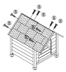
step 3: attach the roofs with screws B.
