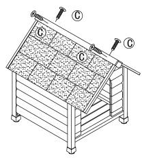
step 4: secure the ridge cap to the roof with scews C.
