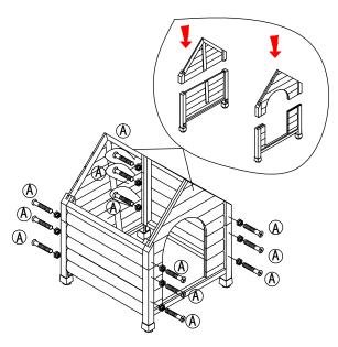
step 1 : secure the front, back and side panels with screws A.
